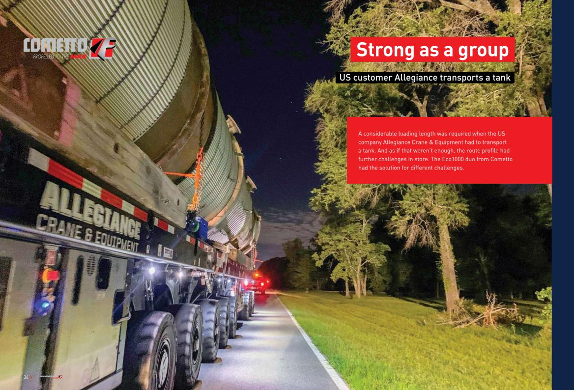
For this mission, the Allegiance specialists coupled a 4-axle and a 6-axle Eco1000 as an "end-to-end" combination. This created sufficient loading length to be able to support the fragile components in the right places. Yet the combination must equally be extremely compact. This is only achieved by integrating the drive units between the axles and modules. In this way, additional loading area is created. That was sufficient for the tank with its length of around 20 meters (67 ft).
