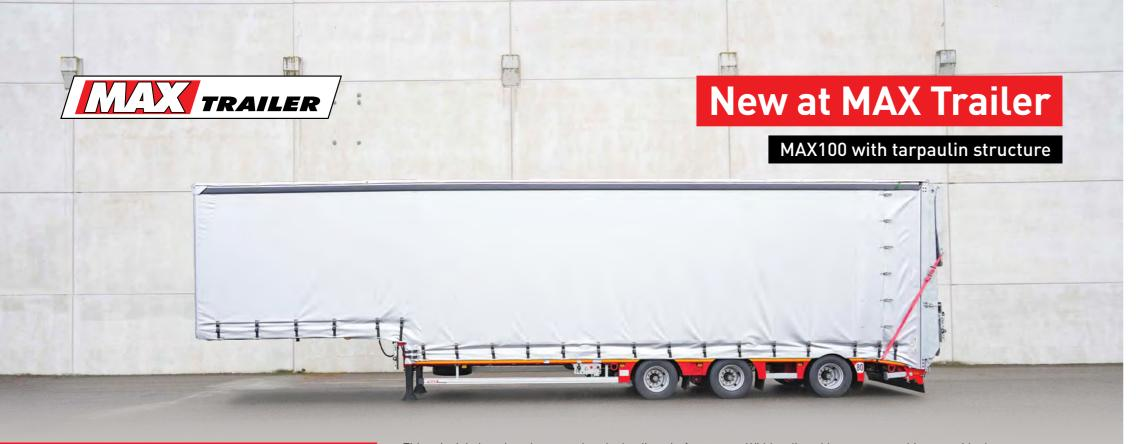
The product diversity at MAX Trailer continues to be developed constantly. The MAX100 semi low loader with friction-steered axle is now also available with a tarpaulin structure.
