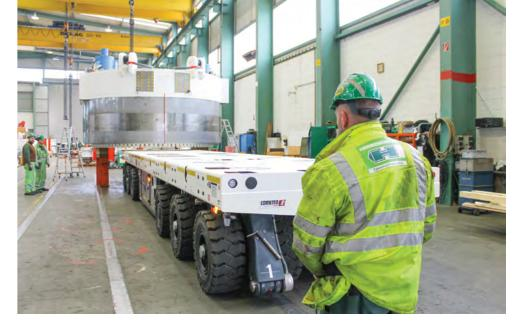
The 6-axle vehicle lines up seamlessly into the work processes at Herrenknecht. Stephan Göggel, Technical Manager of the component factory, says: "With the Eco1000 we are ideally equipped for the in-plant movement of individual components weighing up to 200 tons for our tunnel boring machines."
